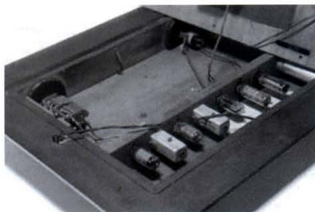
The chassis housing the miniature valves
