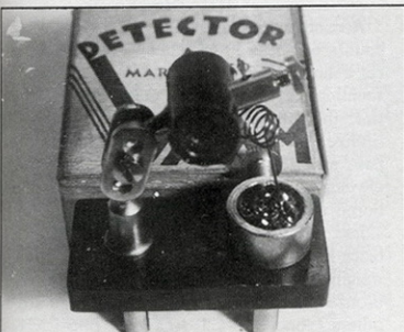
An Italian plug-in galena unit, Detector A Martelleto ("little hammer" or "cat's whisker"), articulo (part no.) 800, ca. 1927.
